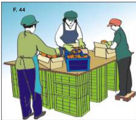
Figure 44: Use a foot platform for small farmers in case of the workstation may be used by many farmers together.
