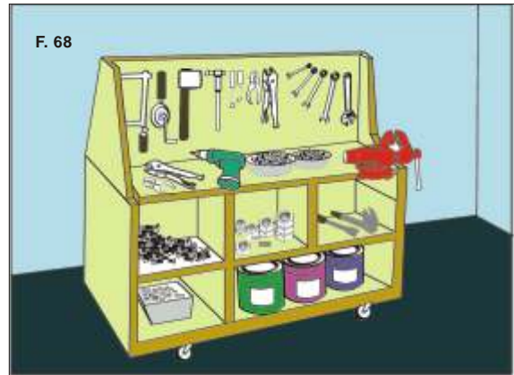
Figure 67: Use a wooden board to fix tool hangers. Mark the shape of each tool clearly and distinctly.
