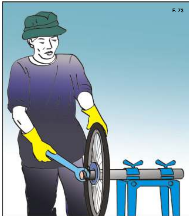
Figure 73: Use a fixture device to hold the naves or rollers when they are detached for repair or maintenance.
