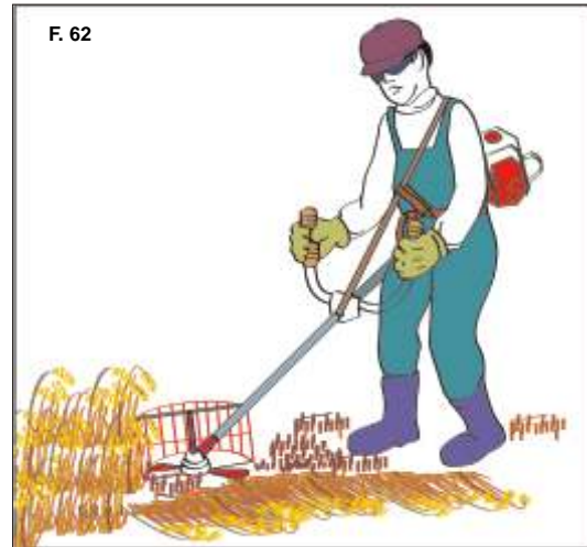
Figure 62: A hand-reaping machine to reduce the workload of your arm and hand muscles. Sturdy hand grips are attached to the machine to secure safe operation.
