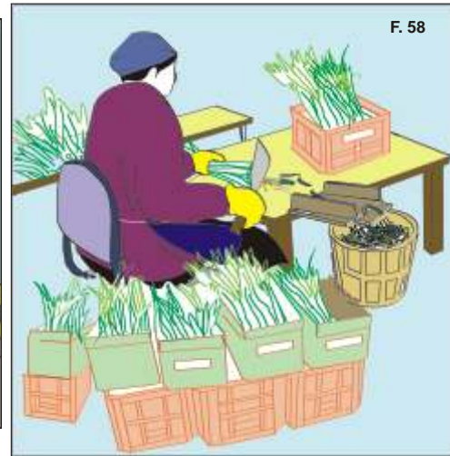
Figure 58: Panniers of raw products and materials are placed within easy reach.
