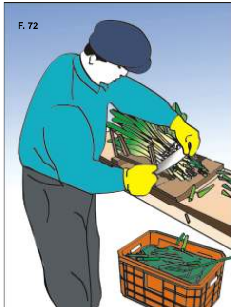
Figure 72: A simple fixture device to hold a bunch of small spring onions.
