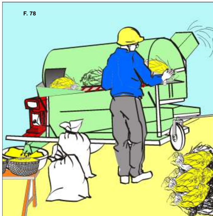
Figure 78 : Feeding device in form of a conveyor which gradually carries the bundles of rice into the threshing machine.
