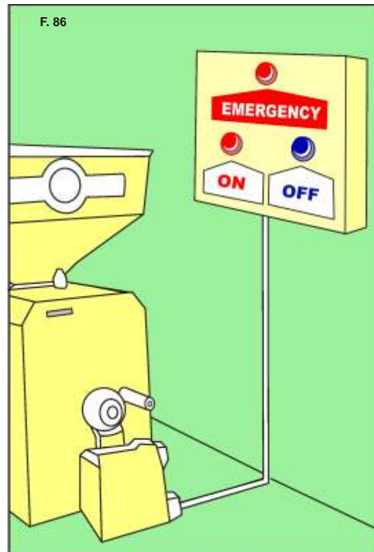
Figure 86: Electrical wires connected to the machine are well protected and clearly labeled.
