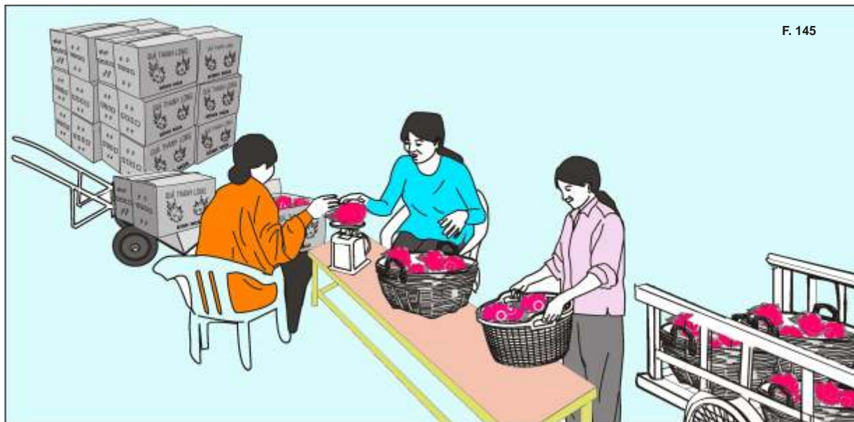
Figure 145 - Move your work items at the same working height. Adjust the working height of work tables and push carts to the same level to minimize the lifting of materials.
